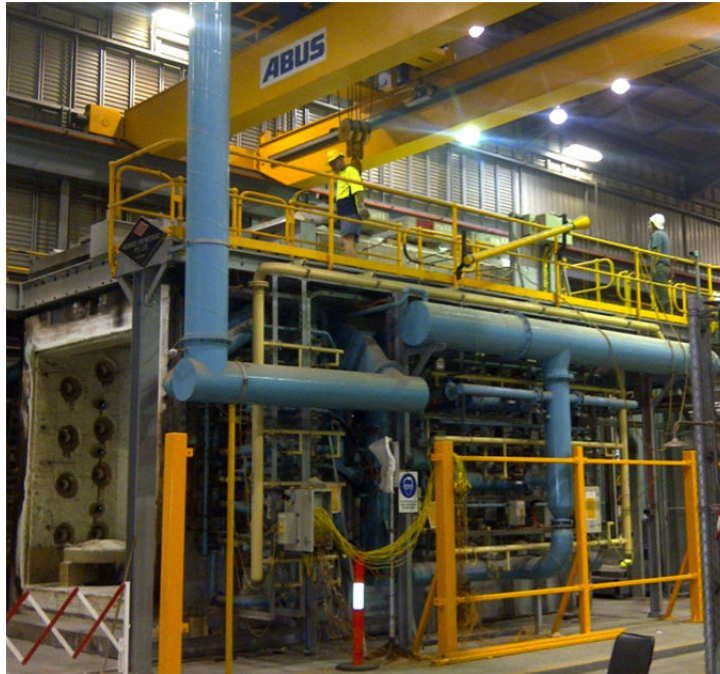
Figure 10: Standard fire testing of geopolymer concrete panel
